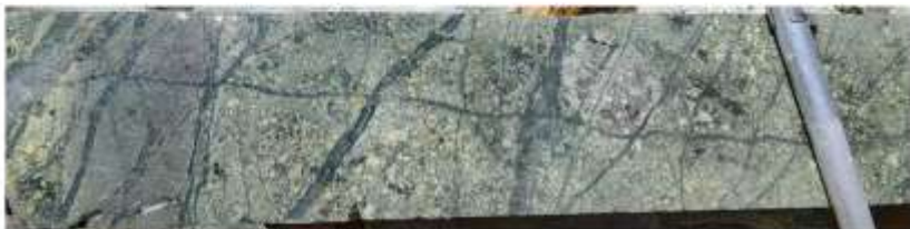
365m: Diorite intrusive breccia with multi pulse quartz vein stockwork.
