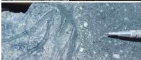
372.72m: Diorite porphyry (amphibole-biotite) intruding Diorite intrusive breccia with quartz stockwork.
