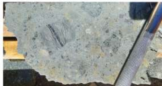
294m: Polymictic pebble dykes including mineralized porphyry clasts and vein clasts.
