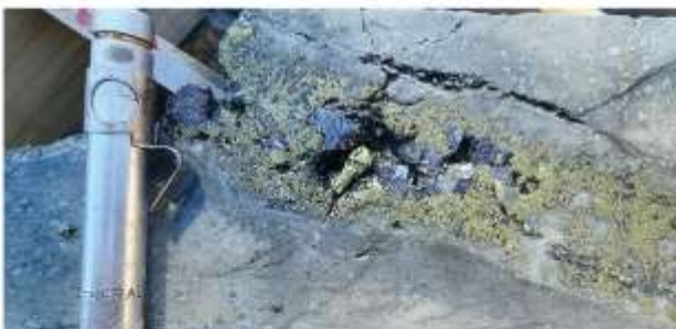
163m: Quartz Diorite Porphyry with polymetallic veins (Qtz-Sph-Ga-Py-Cpy)
