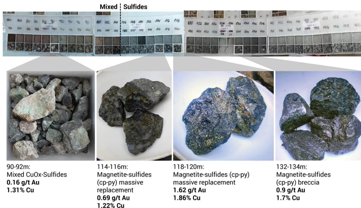
Figure 7: Illustrates the mixed oxide/sulphide and sulphide-only styles of mineralization observed within the RC chips that display abundant chalcopyrite and pyrite.
