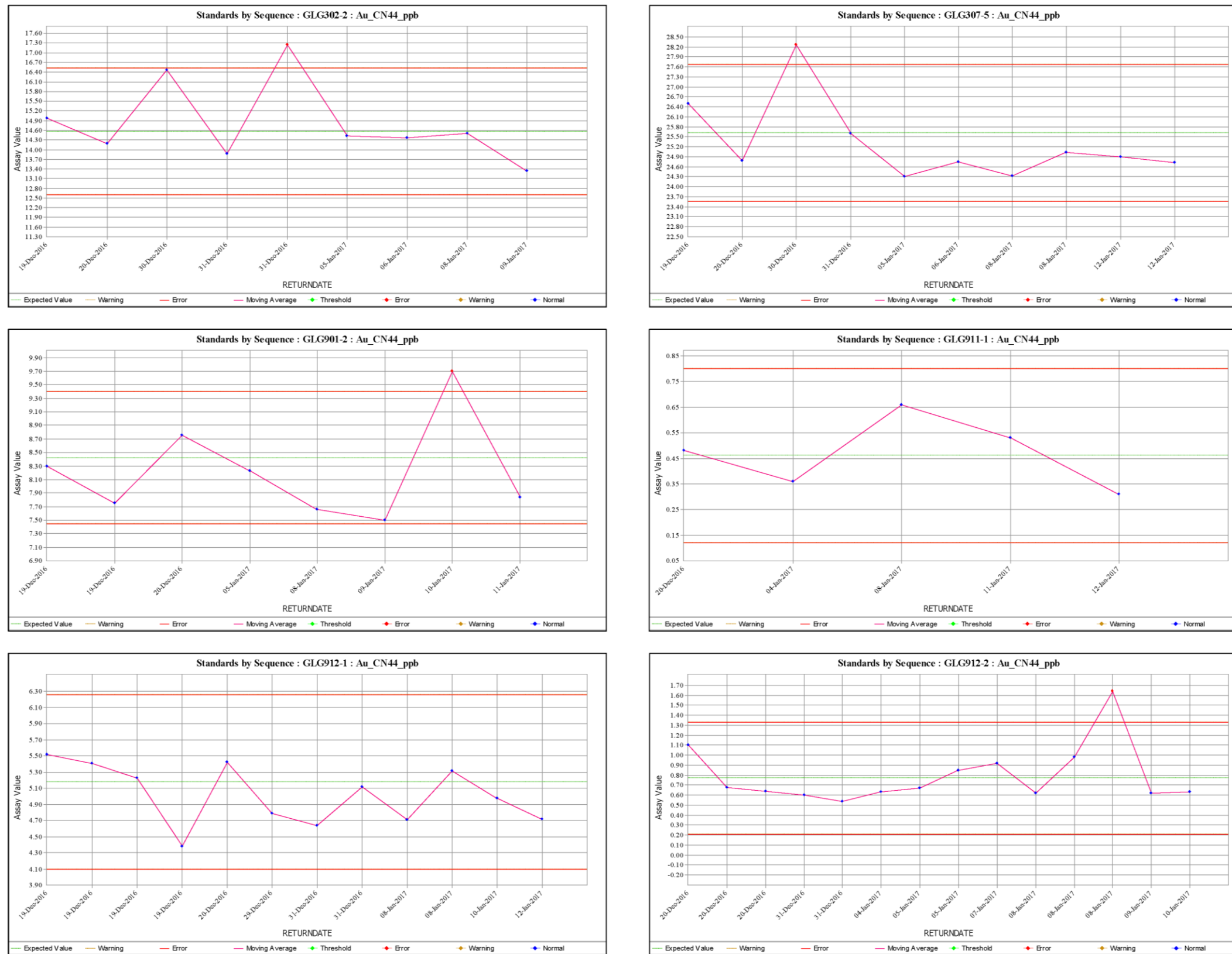
Figure 31. Time plots of standard and blank reference material: GLG302-2, GLG307-5, GLG901-2, GLG911-1, GLG912-1 and GLG912-2 (n=58 total assays).
